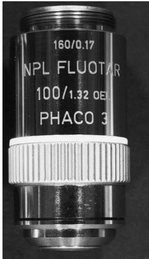
Figure 266. A 100 \times semiapochromat phase-contrast objective intended for use on a microscope with a 160-mm tube length. The numerical aperture of the oil-immersion lens is 1.32, and the lens is meant to be used with a #1.5 coverglass.
