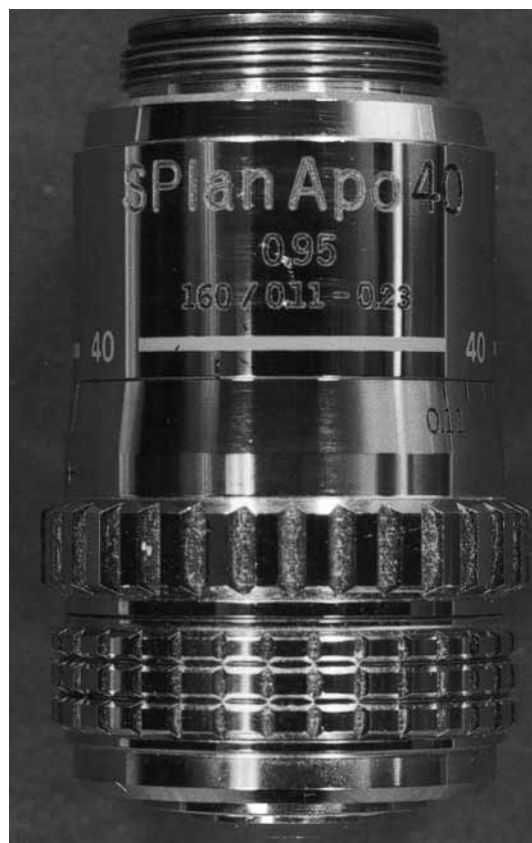
Figure 267. A flat-field 40 \times apochromat objective intended for use on a microscope with a 160-mm tube length. The numerical aperture of the lens is 0.95, and the high-dry lens may be used with #1, #1.5, and #2 coverglasses, as well as for specimens of various thickness. The focusing collar should be adjusted empirically for various specimens, until the image is as sharp as possible.
